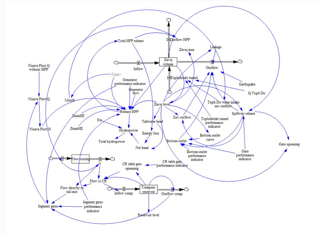
System dynamic model of the Pirot water resources system (a) alongside hazardous models (b).
