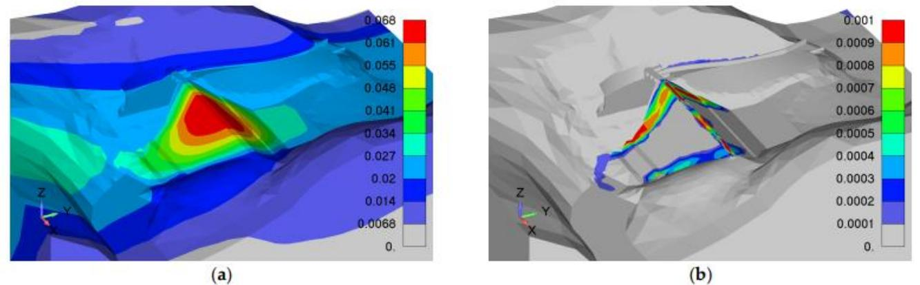
Seismic celeration of the Pirtto water system: (a) total translation and (b) equivalent plastic deformation
