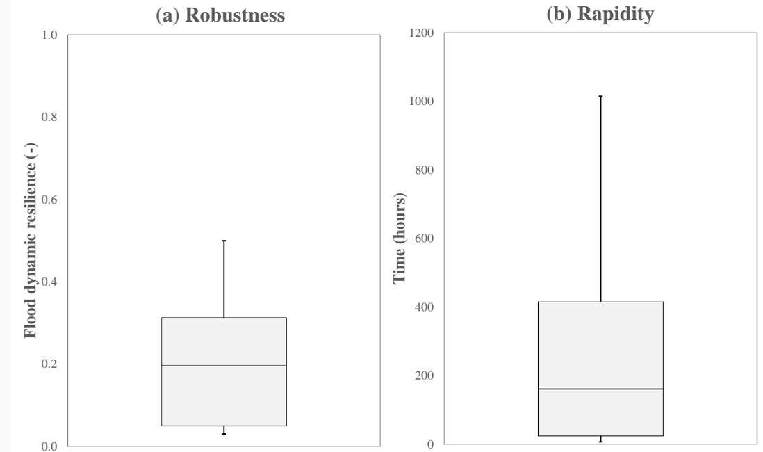
Flood dynamic resilience of the Pirot water resources system using the generated dataset of 1000 simulations: robustness (a) and rapidity (b).
