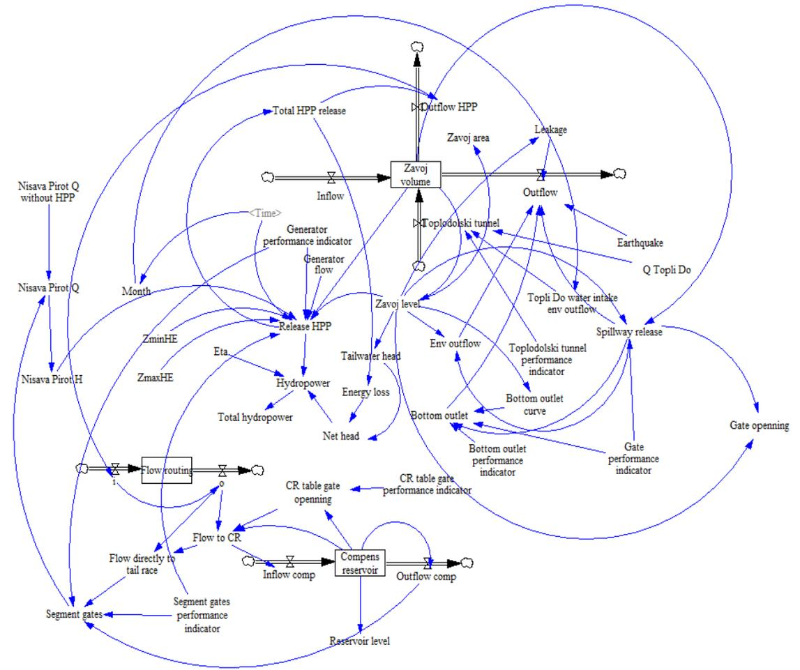
An example: System dynamics model of the Pirot water resources system
